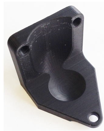
Fig. 6. 3D printed “sled” to hold the projectile.
